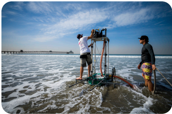
▲ Scripps Oceanography researchers install tide gauges designed to assess wave characteristics and the arrival time of floodwater to upgrade flood alert capabilities and refine the forecasting system.
